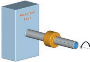
Type 11S Slow rotary movement with type 11S (1 fixed point, 1 side flexible)
