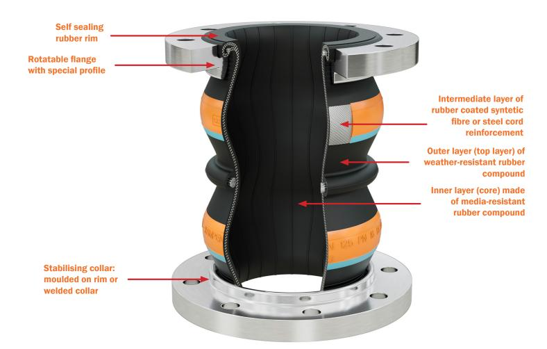
The expansion joints are available in different rubber qualities to ensure the optimum solution for every application. The rubber quality can be recognised by the different colour markings. The additional embossing on the bellows serves to identify the nominal size and the product designation.
